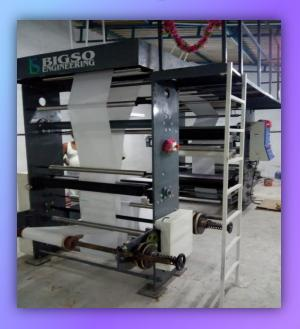
This machine is a special 50 inch width and 50 inch circumference, 4 color Superfast Flexo Printing machine. Here we are giving ladder type for easy handling. We are offering Web Aligner and Automatic lifting handle also for getting best results.
